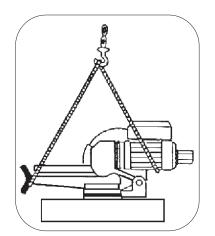
Using proper lifting equipment and lifting straps, raise the circular saw up so its slightly higher than the stand.
