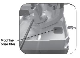
Over the course of the day, the machine will get clogged with swarf and could possibly stop the coolant from running back into the coolant tray. It is best to get into a routine at the end of each working day, or more if its used more frequently to clean any swarf from the machine base casting, filter and vice jaws. Use a soft brush (paint brush or similar) to remove the swarf from the machine at the end of each working day, **NEVER** use compressed air to remove the swarf.
