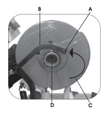
**Caution:** The blade bolt is a left handed thread, meaning to undo it you must turn the bolt clockwise, failing to do this will strip the threads on the blade shaft and possibly snap the blade bolt and will void your warranty.
