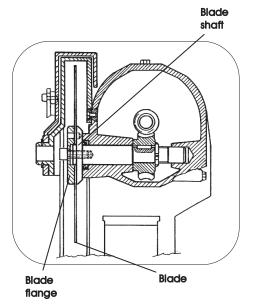
• Once the blade bolt is out, remove the blade flange and then the blade.
