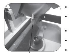
Leave a gap of around 5mm before pressing the handle trigger
