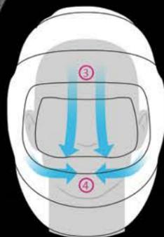
You can even adjust the amount of air coming from the top outlet (3) vs. the two side outlets (4), or choose a blend of both.
