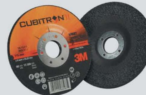
Conventional ceramic grain tends to "plow" through metal, building up heat in both the work-piece and your abrasive. This slows down your cuts and shortens disc lifespan. 3M™ Precision-Shaped Ceramic Grain uses 3M micro-replication technology to form sharp peaks that fracture continuously. This makes for a cooler, self-sharpening abrasive system that slices easily through metal.
